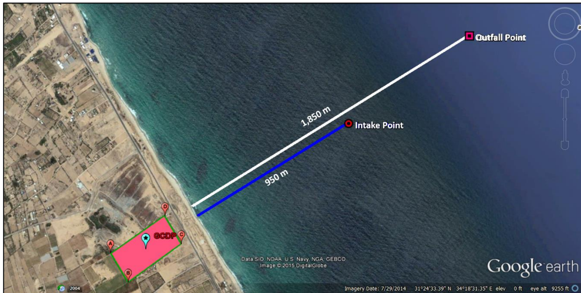
Figure (4.3): GCDP’s intake and outfall systems
